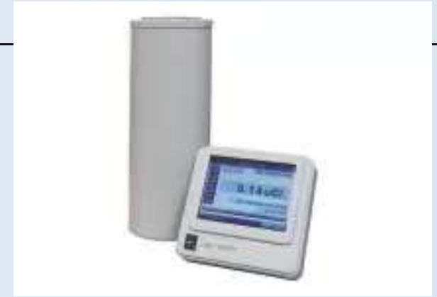
Lead Shield Dose Calibrator Method for ^{99}\text{Mo} Breakthrough Test
